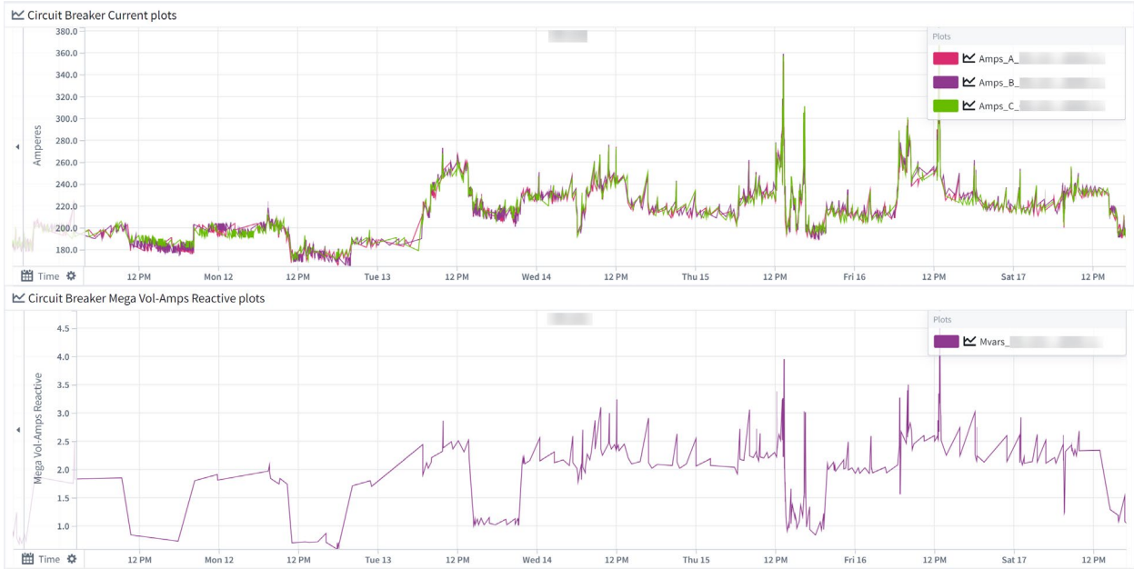
Figure 9: Feeder circuit breaker amps and VAR reactive power
