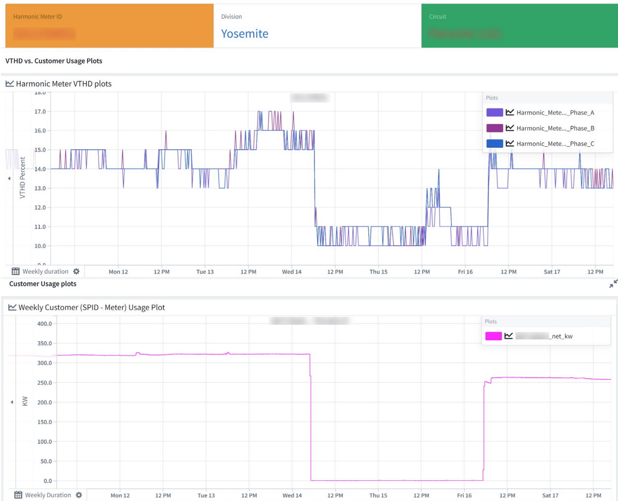
Figure 11: Harmonics correlation - Feeder VTHD and customer demand time series
