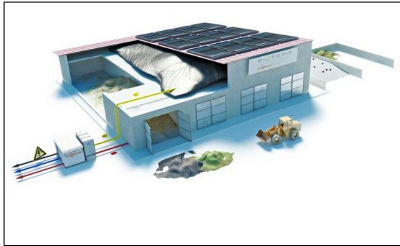
Figure 9: An example of a high-solids fermentation facility (BIOFerm, 2018)
