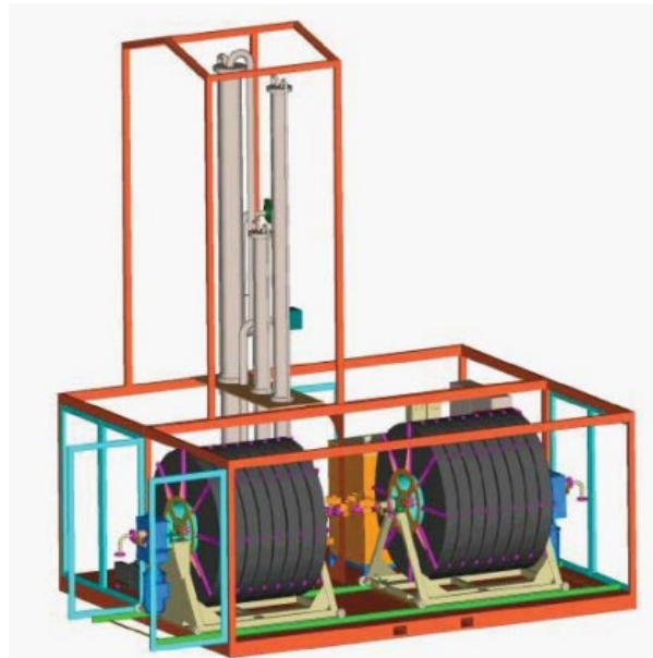
Figure 6 Rotary Coil Water Scrubber (Bauer, 2012)
