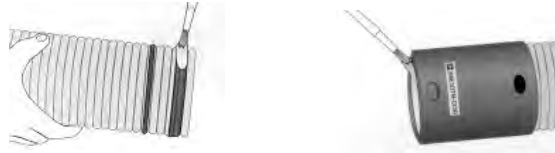
Figure 25 Key-Lock™ Couplers Lubricant Application
