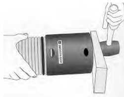
Figure 27 Key-Lock™ Couplers Locked in Place
