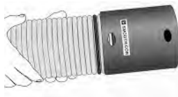
Figure 26 Key-Lock™ Couplers Insertion
